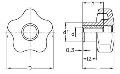
$$\begin{array}{ll} D & = 32 \\ d1 & = 15 \\ d \ 6H = M6 \\ h & = 12 \\ L & = 23 \\ l2 & = 10 \end{array}$$
